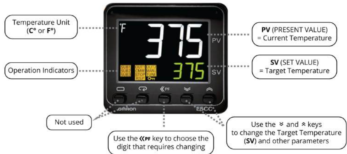
Figure 4 OMRON Digital Temperature Controller
