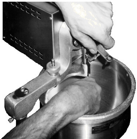
Figure 7 Installing the plunger
