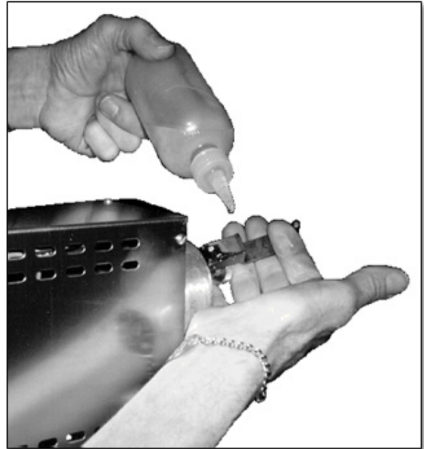
Figure 17 Lubricating connecting rod
