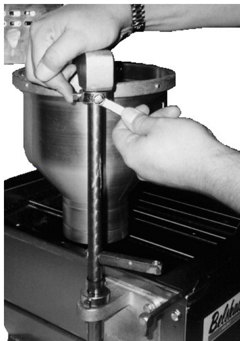
Figure 9 Adjusting the swing of the hopper
