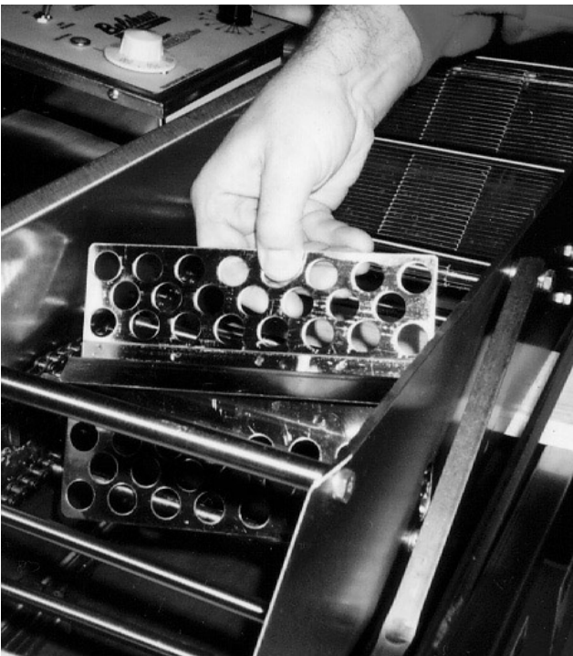
Figure 15 Removing the turner assembly
