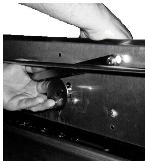
Figure 14 Removing turner cam assembly
