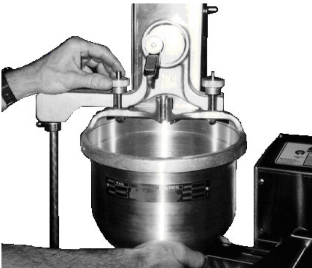
Figure 6 Mounting the hopper
