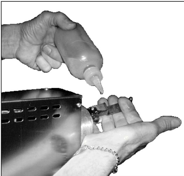
Figure 2-1. Lubricating the Connecting Rod.
