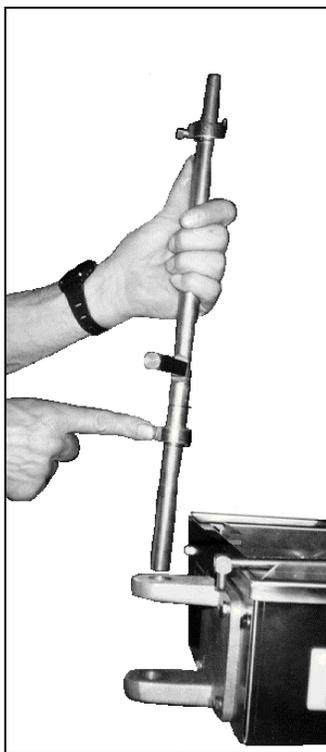
Figure 1-3. Inserting the Swing Column.
