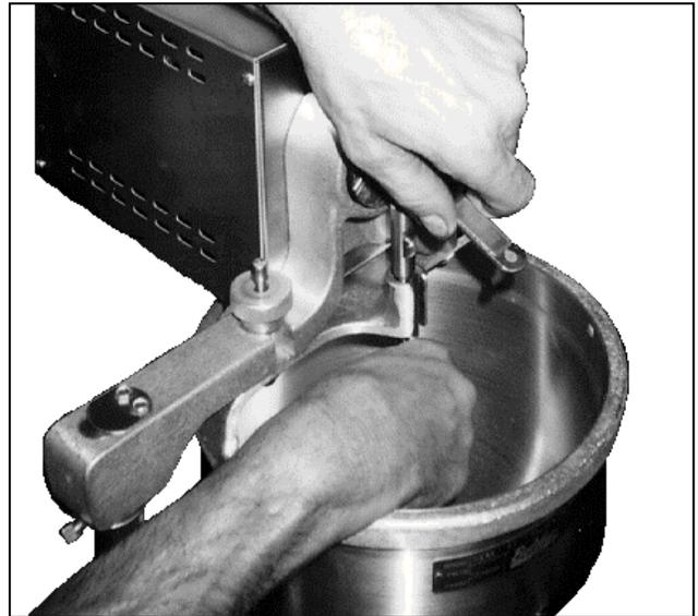
Figure 1-7. Installing the Plunger.
