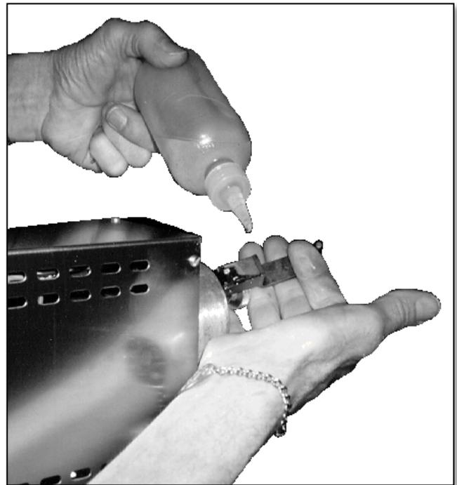
Figure 6 Lubricating the Connecting Rod.
