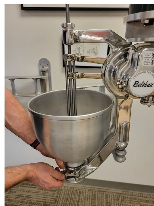
21 Close and tighten cylinder clamp
