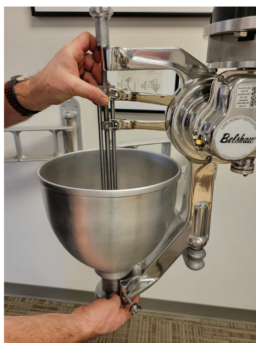
19 Install hopper cylinder and plunger onto Type F
