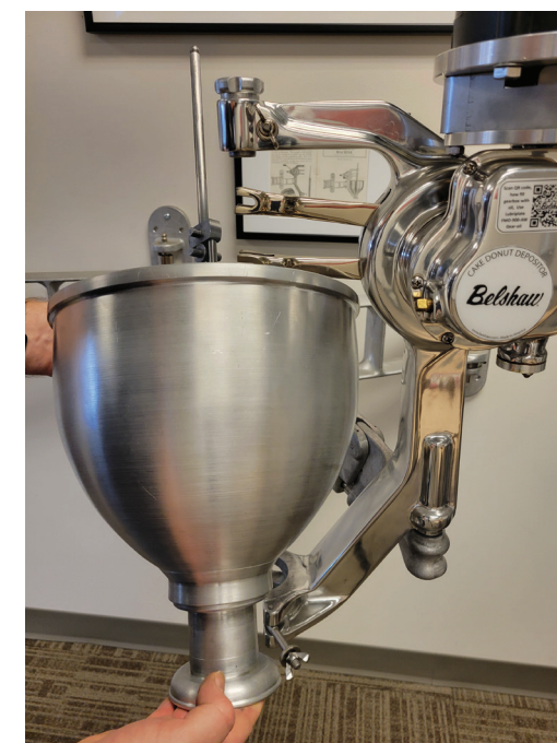
18 Install plunger into cylinder and hopper
