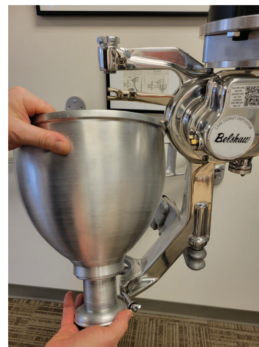
17 Push the hopper tightly onto cylinder
