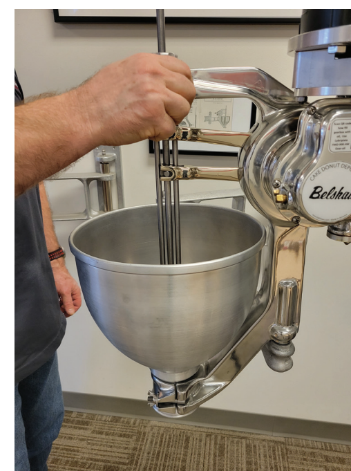
22 Tighten crown bearing clamp
