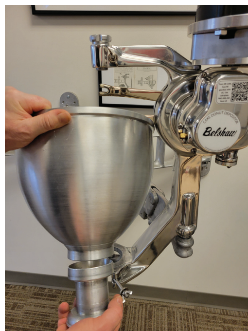
16 Install hopper onto cylinder
