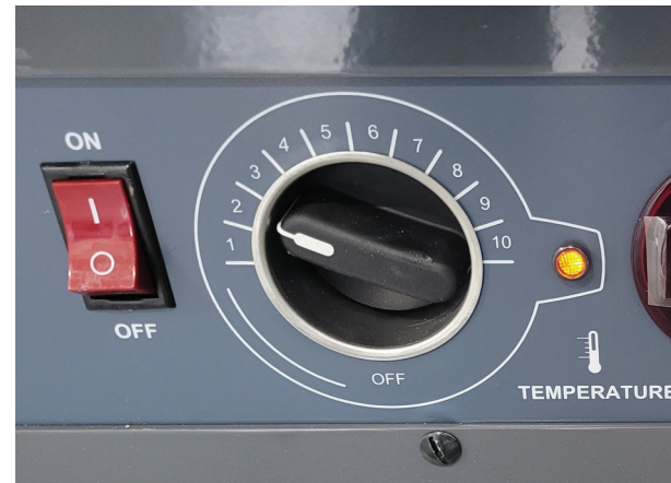
29 Adjust the temperature dial at 2.5 to 3 for 95° - 100°F
