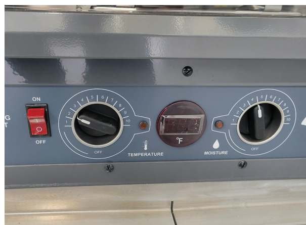
34 Turn the proofer power switch to the OFF position when finished
