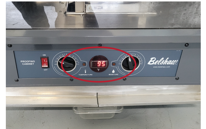
32 Indicator lights will turn off once the temperature and humidity are reached
