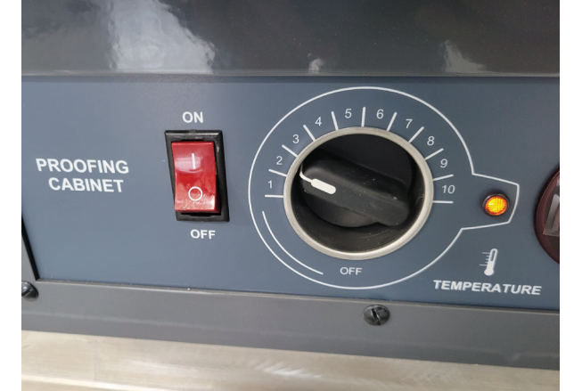
27 Turn the proofer power switch to the ON position
