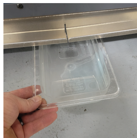
35 Empty the drip pan when finished
