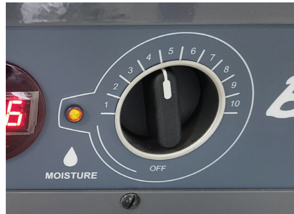
30 Adjust the moisture dial at 4 to 5 for 60% - 70% humidity
