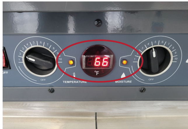
28 The temperature and moisture indicator lights will turn on
