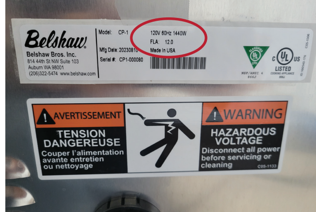
23 Check the data tag on the back of the proofer, verify voltage before using
