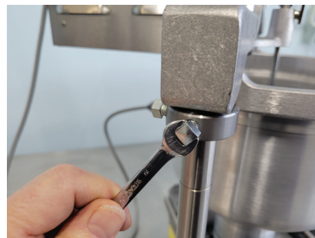
37 Loosen cutter head set screws with 5/16 wrench (x2)
