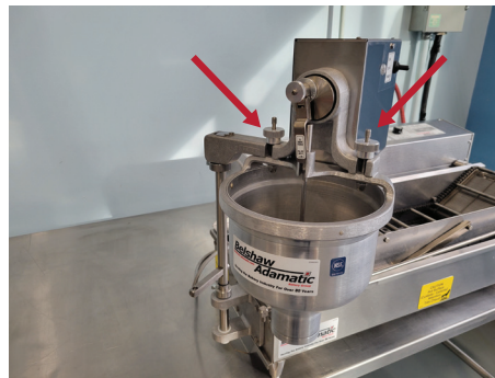
26 Tighten hopper mounting nuts
