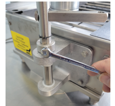
29 Loosen set screw adjust with 5/16 wrench
