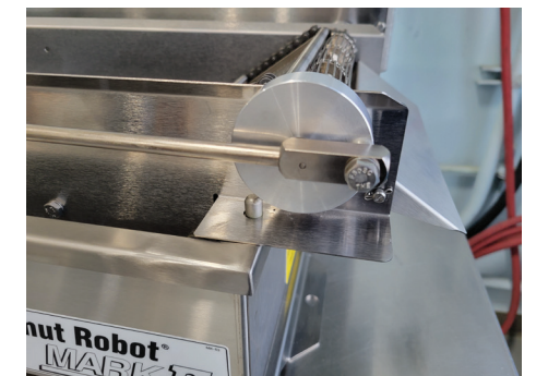
41 Stop conveyor with connecting rod to right
