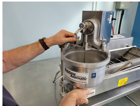
25 Install hopper onto cutter head
