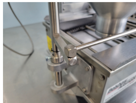
38 Attach connecting rod to swing arm
