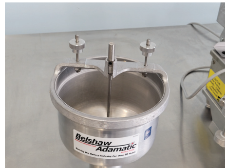
24 Install plunger into hopper
