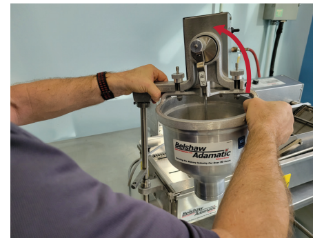
27 Lift and swing hopper over conveyor
