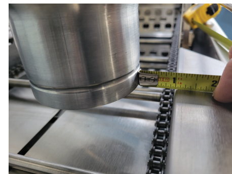
39 Adjust hopper 1 inch from side panel
