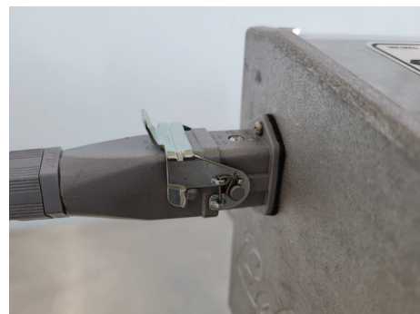
30 Plug cutter head into fryer
