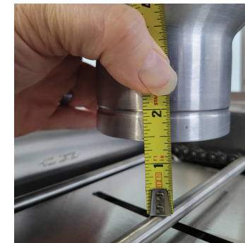
28 Adjust hopper height to 1 3/8 in. with tape measure
