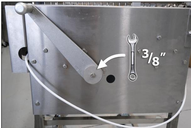
**Figure 3:** Removing the Lift Handle.
