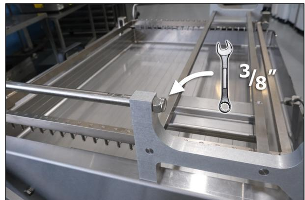
**Figure 4:** Removing the Tray Retainer Handle.
