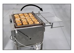
Fig. 10: Tray Retainer in OPEN position.
