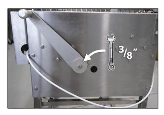
Figure 3: Removing the Lift Handle.
