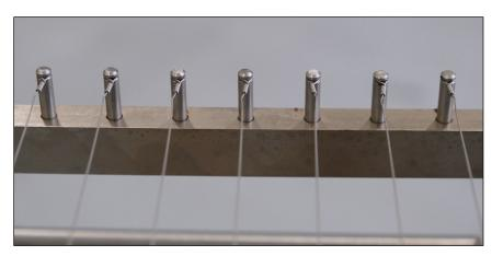
Figure 1: Looped end of wire
