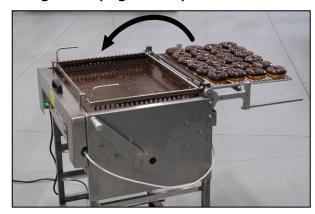
Figure 15: Rotate the Donut Retainer frame to CLOSED position.
