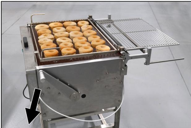
**Figure 11:** Push down on the Lift Handle to ice donuts
