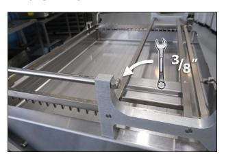
Figure 4: Removing the Tray Retainer Handle.
