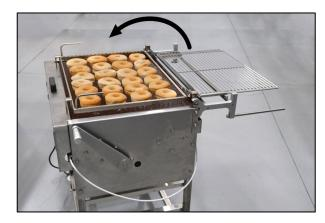
Figure 12: Rotate the Donut Retainer Frame back into the CLOSED position.
