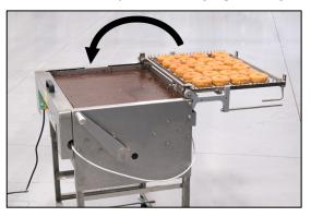
Figure 8: Rotate to CLOSED position.
