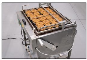
Figure 9: Place Donuts over icing pan.
