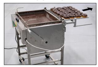
Figure 16: Remove the screen or tray of donuts.
