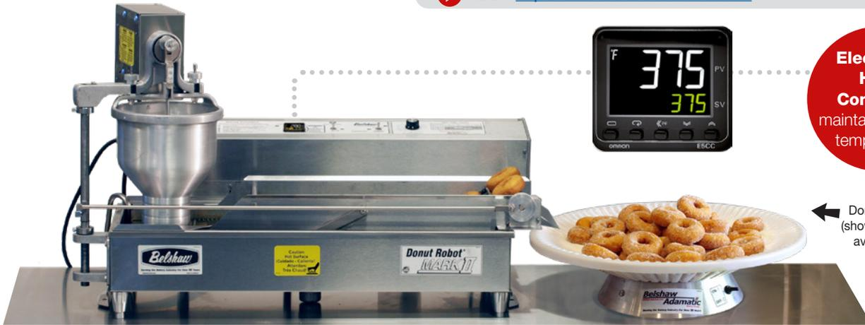
**Electronic Heat Controller** maintains steady temperature
