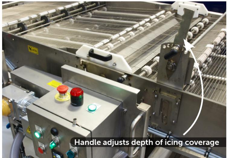
Handle adjusts depth of icing coverage
