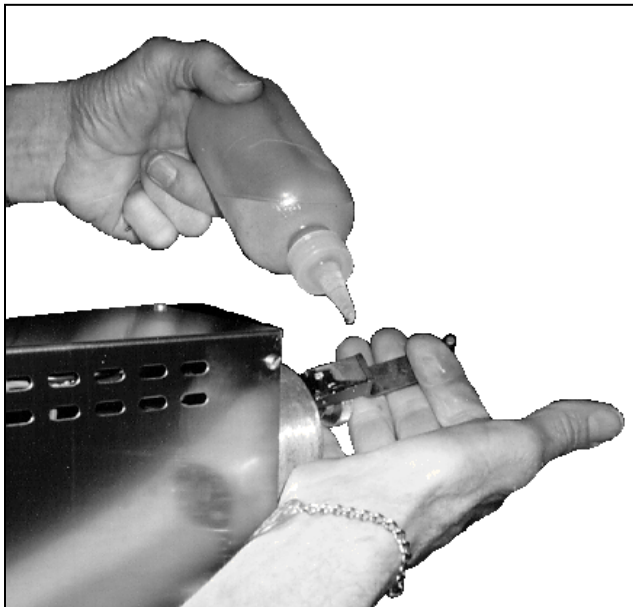
Figure 2-1. Lubricating the Connecting Rod.
