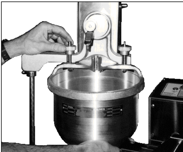
Figure 1-6. Mounting the Hopper.
