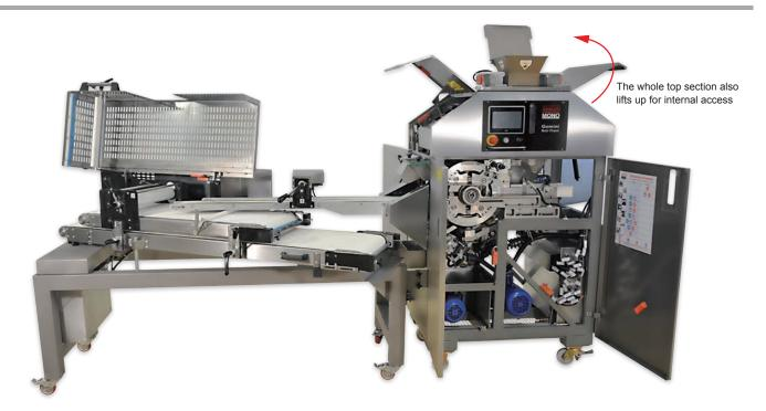
MONO's Gemini Two-Pocket Roll Plant and Roll Forming Unit have been designed to provide direct and unimpeded access to all areas, making the regular cleaning process as quick, simple and hassle-free as possible.
