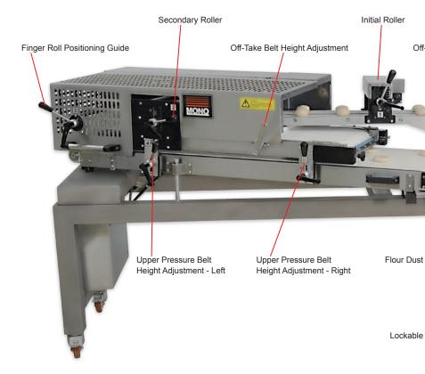
The specially designed Roll Forming Unit truly transforms the roll plant into a highly versatile roll production factory enabling a huge variety of round, hamburger, petit pain and hotdog / finger rolls to be created from the one machine providing genuine product flexibility.
