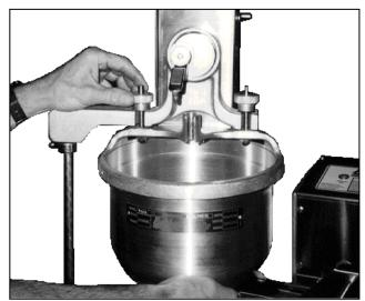
Figure 1-6. Mounting the Hopper.
