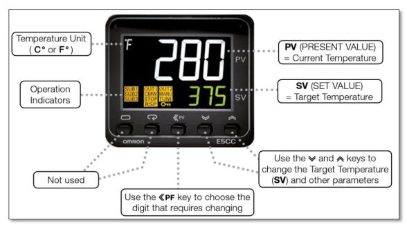
Figure 1.2, Temperature controller
