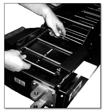
**Figure 5 Removing the Drop Plate**
