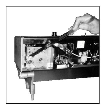
Figure 2-3. Lubricating the Drive Gears.
