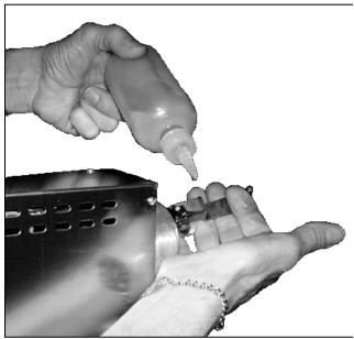
Figure 2-1. Lubricating the Connecting Rod.
