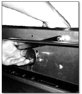
Figure 3 Removing the Turner Cam
