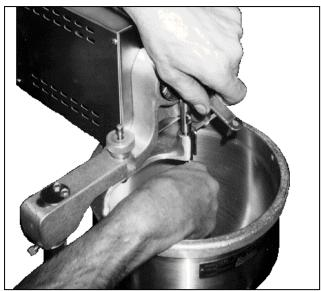
Figure 1-7. Installing the Plunger.
