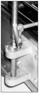
Figure 1-4. Connecting the Swing Connecting Rod.
