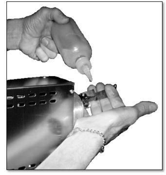
Figure 6 Lubricating the Connecting Rod.
