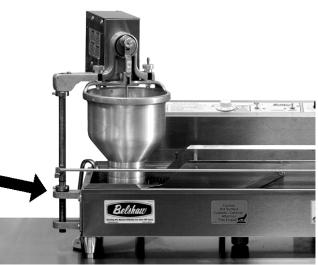
Figure 2-2. Lubricating the swing column.
