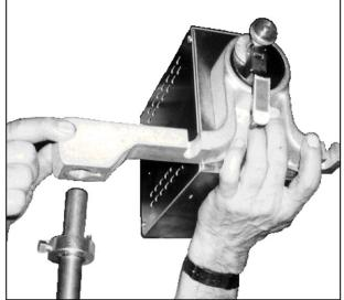
Figure 1-5. Mounting the cutter head.
