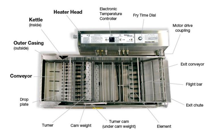
Figure 1.1. Donut Robot<sub>®</sub> Mark VI
