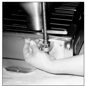
Figure 1-8. Adjusting the Height of the Hopper.
