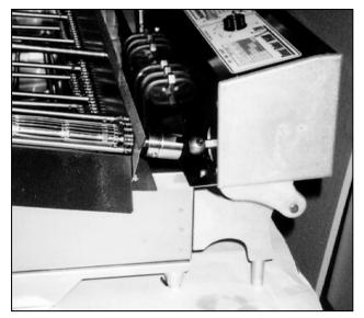
Figure 1-2. Joining the Couplings.
