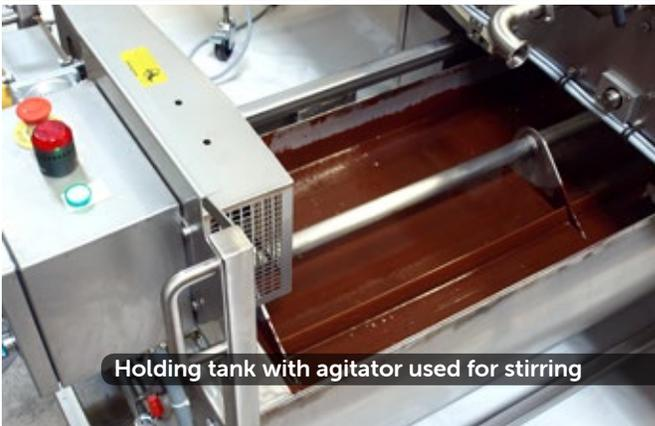
Holding tank with agitator used for stirring
