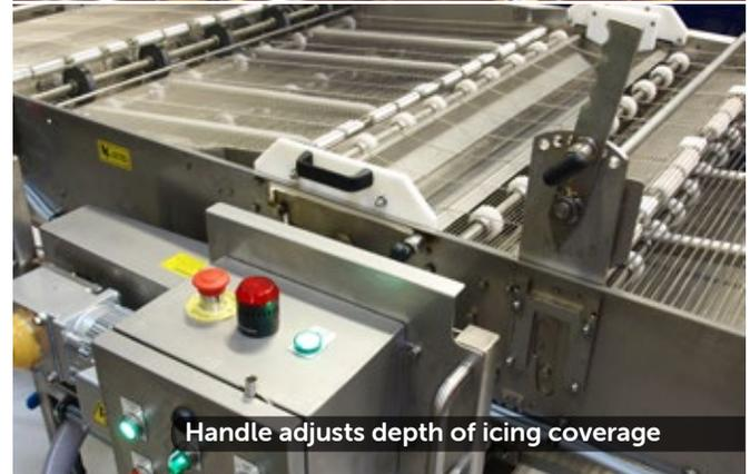
Handle adjusts depth of icing coverage
