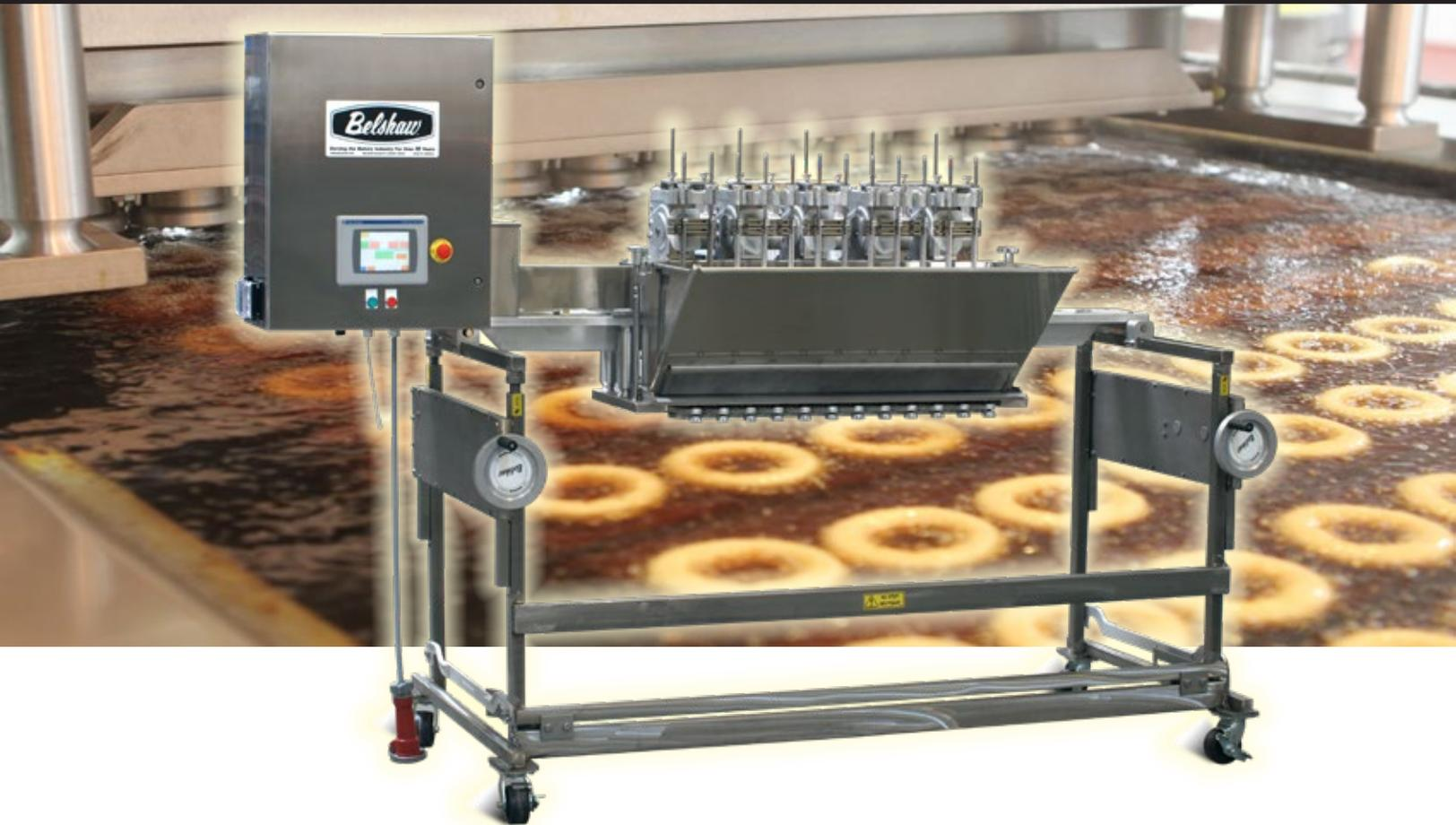
Belshaw has developed a High-Speed Multi-Spaced version of the Belshaw MultiMatic, which has long been the industry standard for cake donut production. It is a proven reliable machine that can produce a wide variety of cake donut products and sizes, offers quick product changeover and is easy to operate and easy to clean. In addition to these features, Belshaw can now offer production rates of 100+ cuts-per-minute, at 20 cuts across the fryer.
