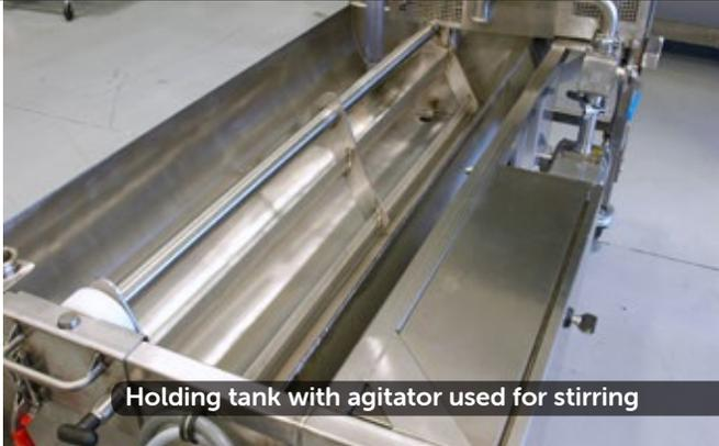
Holding tank with agitator used for stirring
