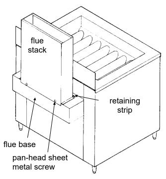
Figure 1-1. Installing the Flue Stack.
