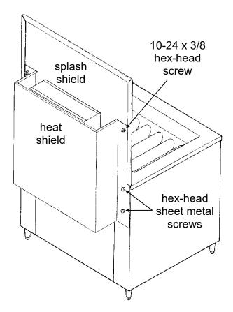
Figure 1-2. Installing the Heat Shield and Splash Shield.
